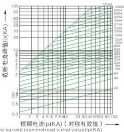
"gG"熔断体的截断电流特性曲线 Breaking current characteristics curve of "gG" fuse links
