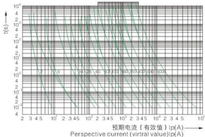
"gG"熔断体的时间—电流带 Time - current range of "gG" fuse links
