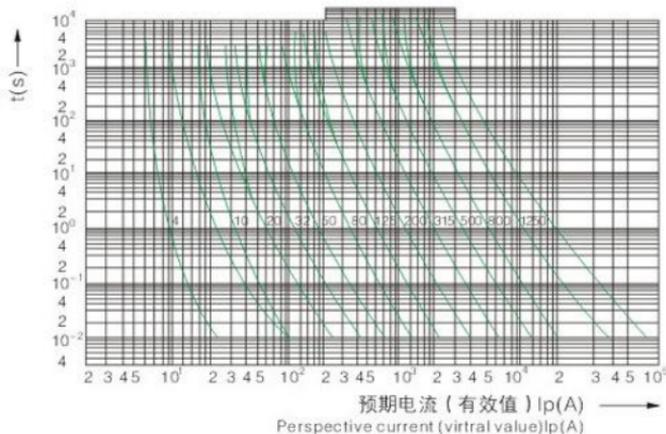
"gG"熔断体的时间—电流带 Time - current range of "gG" fuse links
